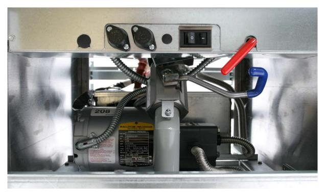
The blue handle drains the frypot. The red handle operates the filter pump.
